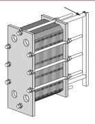
7 Mark the plate assembly on the outside by a diagonal line.
