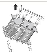
6 Lower the heat exchanger into a horizontal position and place it on the floor.
