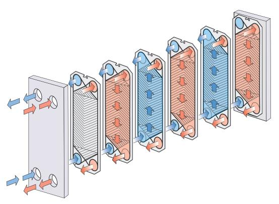
Figure 2: Example of a single-pass set up.
