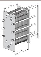
Loosen and remove the locking bolts. Identify them according to *Bolt configuration* on page 33.
