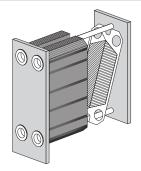
If the plate pack has been marked on the outside, check this (see step 7 on page 35 in Opening on page 33). If the plates are correctly assembled (A/B/A/B etc.), the edges form a "honeycomb" pattern, see picture.
