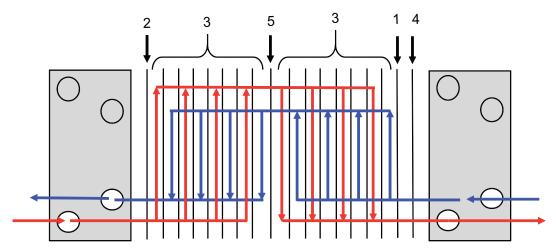
Figure 3: Example of a multi-pass set up.
