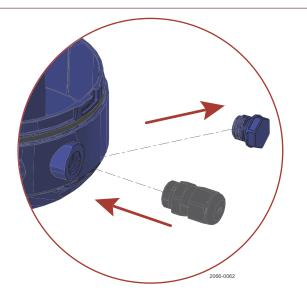
2 Fit the black bushing in the relevant hole in the valve yoke.
