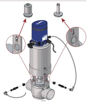
Position the valve so that the mechanical target is in front of the sensor by manually controlling solenoid valve two.
