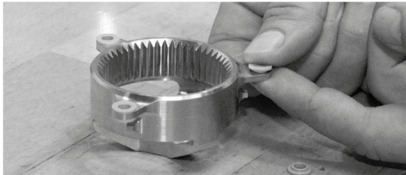
2. Mount bearing for body (13.3) on the gear frame (13.2). Use Drift (TE81B139) and hammer to apply pressure.
