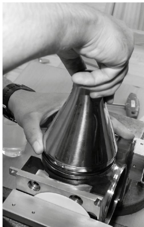
7. Mount assembled planet gear in the gear ring (13.2)
