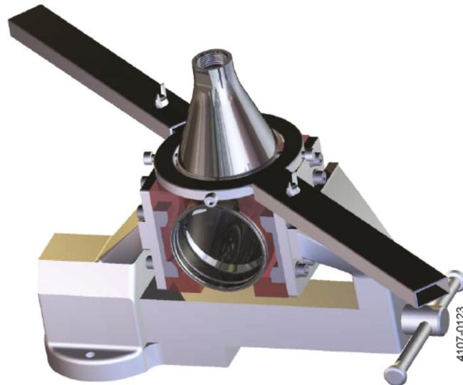
11. Tighten the stem nut (4) until you feel a stop and then tighten a bit more (the stop you feel are two surfaces connecting).
