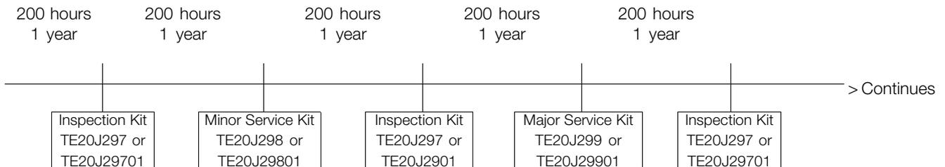
It is recommended to inspect the Alfa Laval Toftejorg SaniJet 25 after every 200 running hours or after 1 year to ensure the conditions of the machine is acceptable. During the inspection it is recommended that the inspection kit is used in order not to compromise the hygienic state of the machine.
