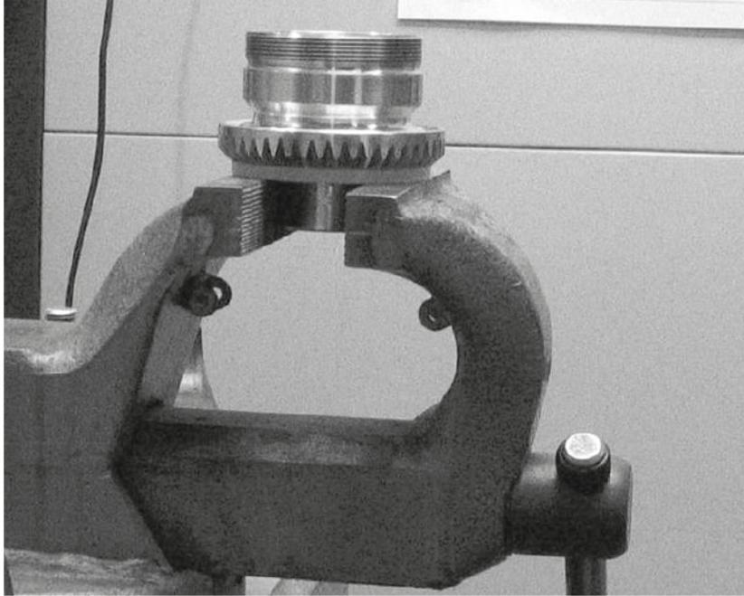
3. Place the ball retainer with balls (5) onto the ball race on the stem (8).
