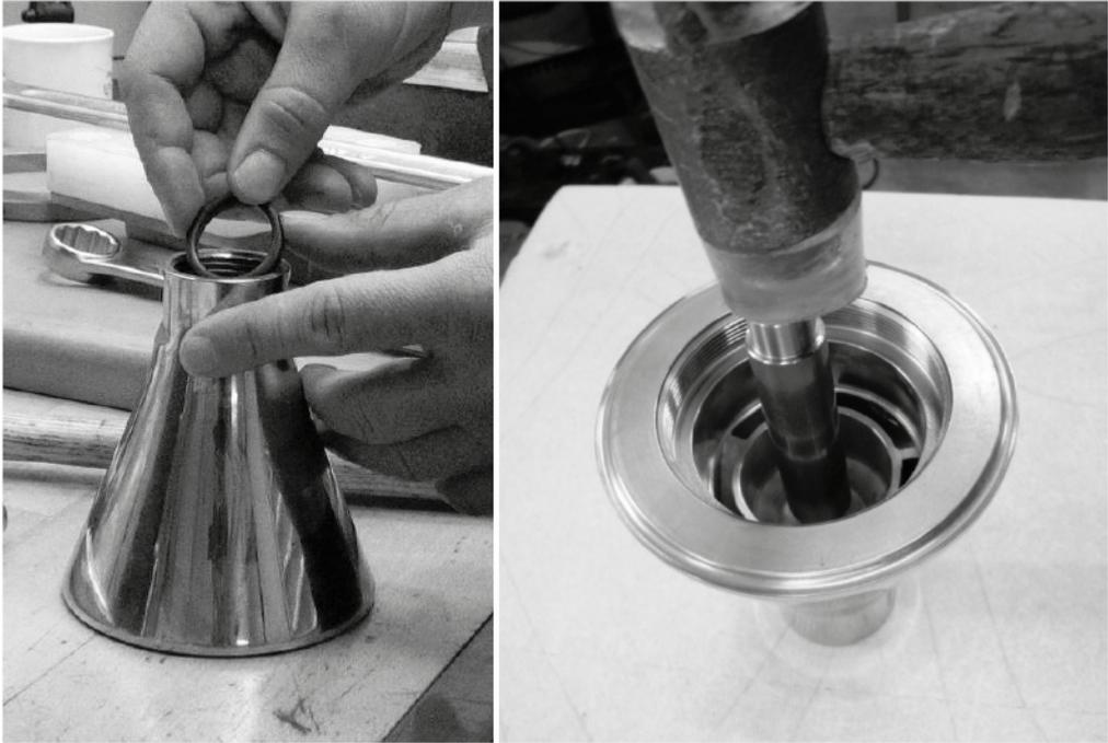
10. Push out bushing (1.2) from the top of the cone using the drift (TE81B139)
