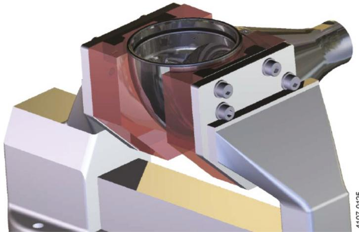
16. Preparation before mounting the assembled lower parts on body (13.1): It is recommended to grease the body thread with food graded/FDA compliant grease. The grease reduces the risk of galling in threads. The grease is enclosed between the O-rings and, therefore, it will not come into contact with the cleaning media.
