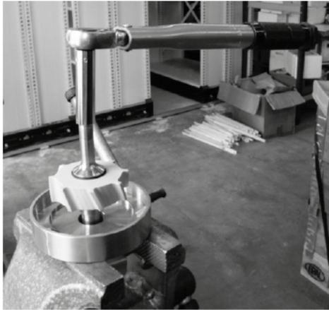
5. Screw the shaft end (3.4) into the turbine shaft (3.1) using the torque wrench (TE81B156) and NV9 spanner socket (TE81B158). Tighten with torque of 10-12 Nm.
