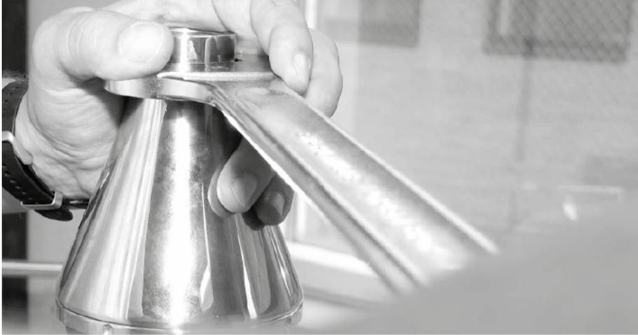
4. Loosen the cone (1.1) by hand while lifting the cone vertically and finally remove the cone (1.1)
