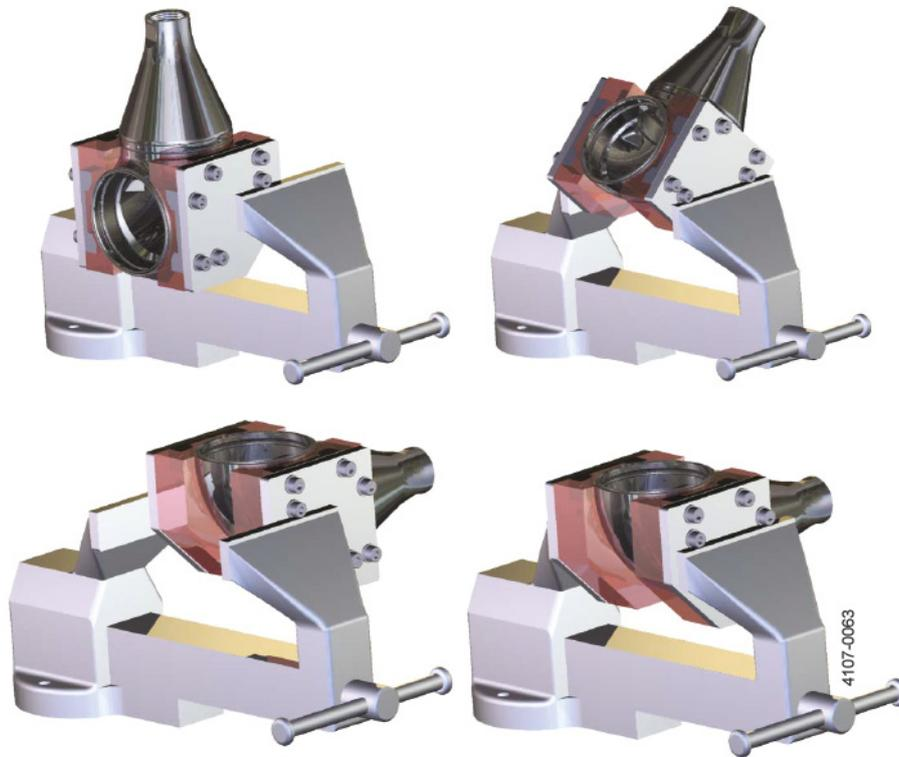
12. Lower the ring key (TE20J393) around the hub nut (15) and tighten the 4 screws (by hand only) symmetrically on the 4 hygienic recesses in the hub nut (15). Loosen the hub nut (15). **Left handed thread.** When hub nut is loosened unscrew with hands.
