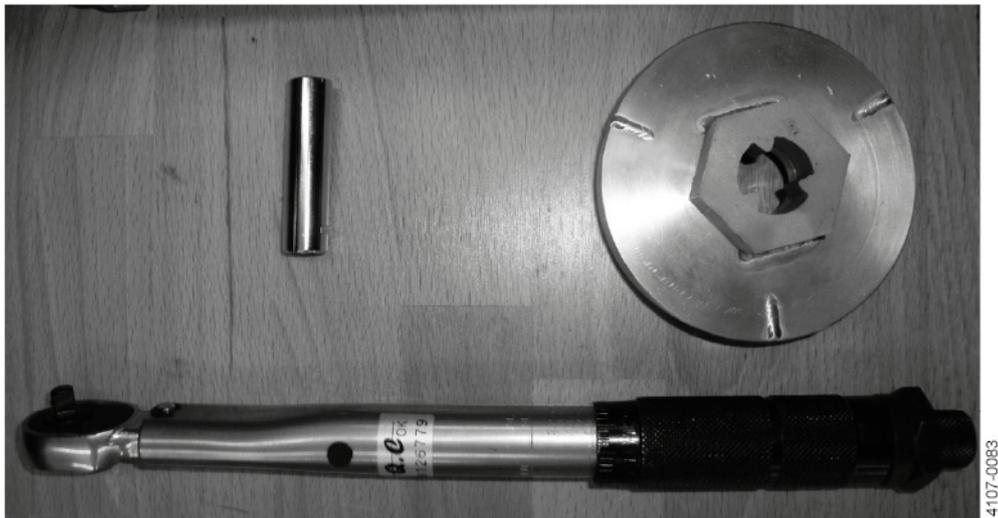
1. Mount the impeller turbine fixture (TE20J392) in bench vise. Loosen the shaft end (3.4) using the torque wrench and NV9 socket long (TE81B156 + TE81B158) and unscrew with hand.
