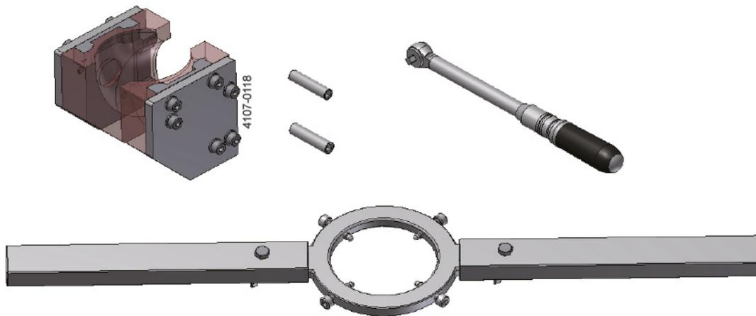
1. Put the two fixtures (TE20J386) around the house and slide the assembly between the jaws of the bench vise. Let the bolt ends slide on-top of the jaws. With the SaniJet 25 centred between the jaws tighten the bench vise.
